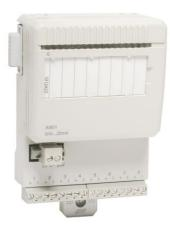
The AI801 Analog Input Module has 8 channels for current input. The current input is able to handle a short circuit to the transmitter supply at least 30 V d.c without damage.
